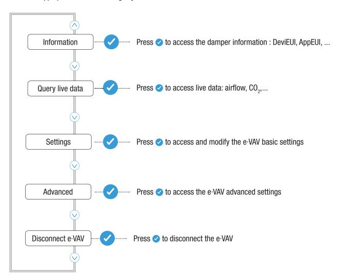
The remote control allows you to modify all the e-VAV parameters : airflow,  $CO_2$  level, ..... In order to modify parameters, the remote control has to be wirely plug into e-vay.
