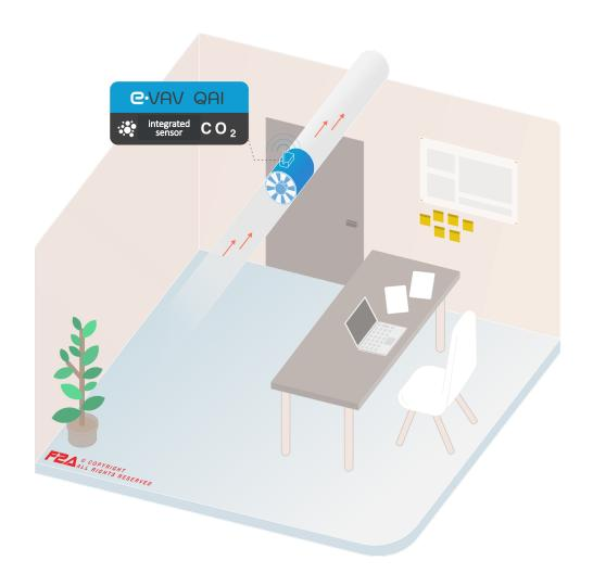
The **e-VAV QAI** damper in the exhaust is controlled by the  $CO_2$  measured by its integrated sensor. The damper is factory set with minimum and maximum airflow and  $CO_2$  values.
