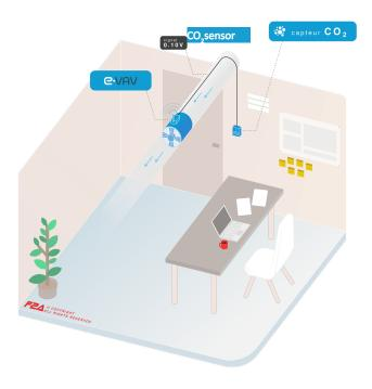
The damper is controlled by a  $0..10\,\mathrm{V}$  signal from a room  $\mathrm{CO}_2$  sensor which itself measures in real time the  $\mathrm{CO}_2$  concentration and sends a  $0..10\,\mathrm{V}$  signal to the damper to adapt the airflow rate.
